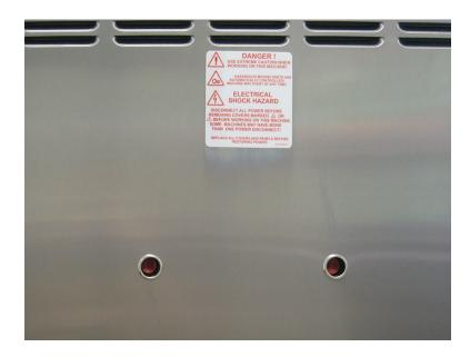
If the mix gets too cold, the reset button will "trip" to protect the beater motor. This could be caused by insufficient mix in the freezing cylinder. If this occurs, inspect the feed tube to verify that it is properly assembled.
